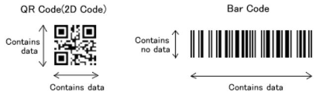
Figure 5. two-dimensional QR code vs one-dimensional barcode [9]
