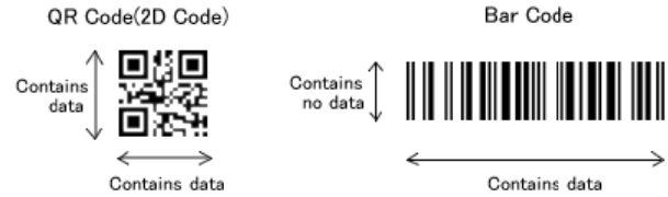
Figure 3. Two-dimensional QR code vs one-dimensional barcode
